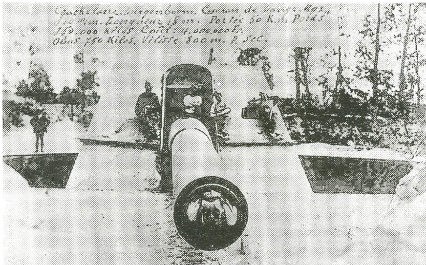
Above: The Leugenboom gun Long (Lange) Max of 38 cm calibre (14.5 inch approx). Note the figure squeezed into the muzzle.
