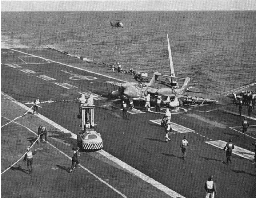
The Flight Deck parties ready for any eventuality as a Sea Vixen with a faulty wheel assembly makes the only 'barrier landing' of the Commission
